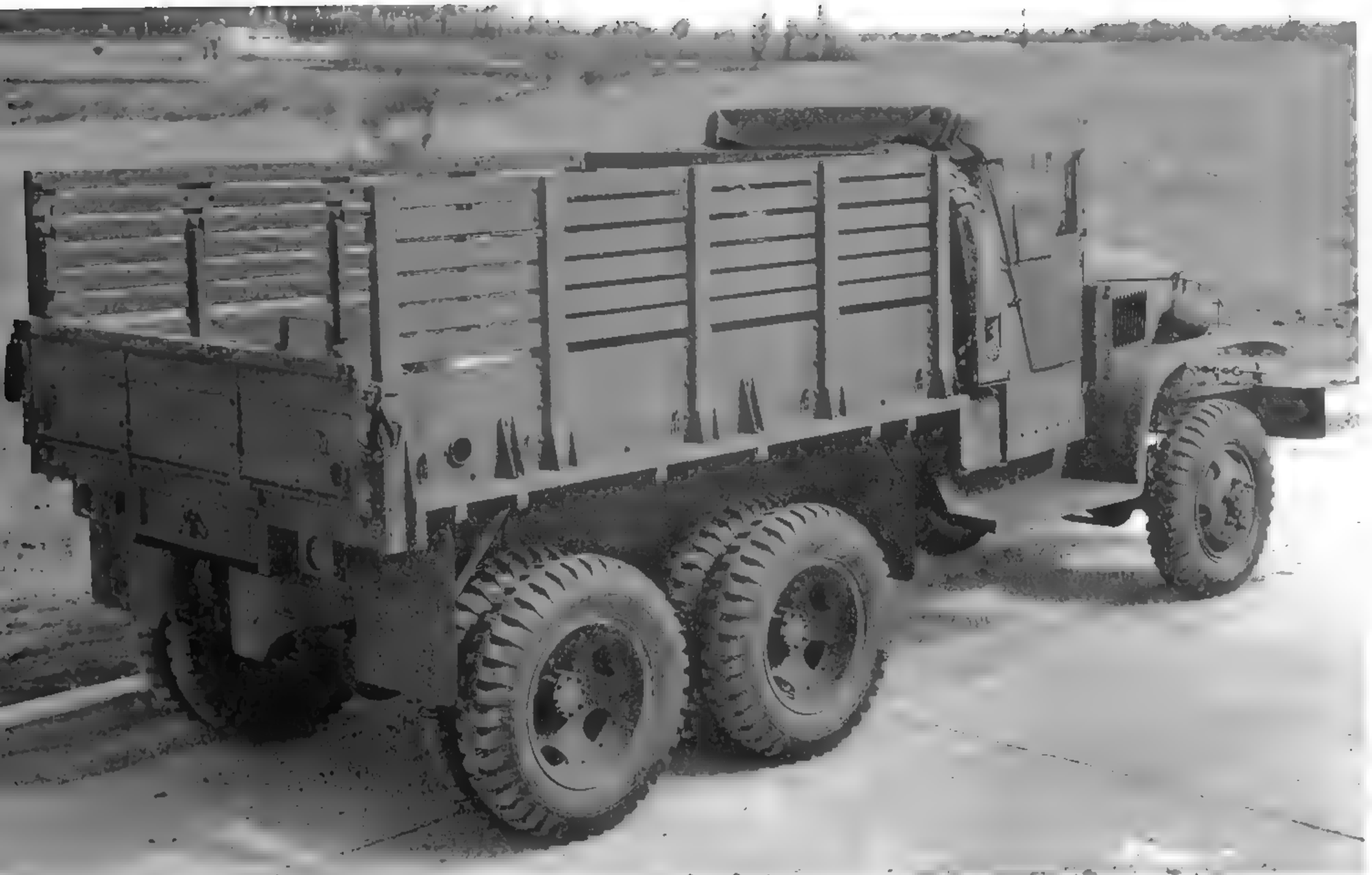
As the war continued, the closed cab of the CCKW-352 gave way to the open cab, and the steel cargo bed was replaced with one of wooden construction, as seen here. (Photo courtesy of Bryce Sunderlin collection)
